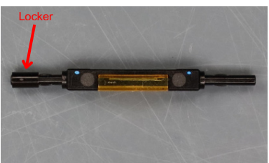
Step 6: Add a locker (black) onto one side of the mechanical splice, keeping it near the tip.
